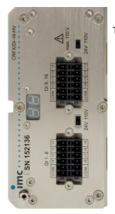
The common reference ground of each 4-bit group is located at LCOM
