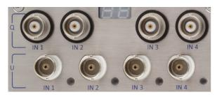
The connection is made via eight BNC sockets, four of which are for voltage measurement or optionally for ICP ( $\mathbf{U}$ ) and four for charge measurement ( $\mathbf{Q}$ ). The connections are labeled accordingly: U or Q
