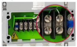
for the thermocouple variant: HVBOX-8-T-10M as an example, two wires are enlarged left + and right - for the fourth thermocouple
