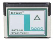
CFast is based electrically on the SATA Standard, while CF is based on the parallel IDE-ATA, so that the former offers significantly higher transfer speeds.
