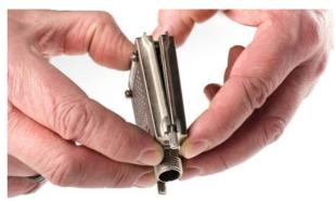
ACC/DSUBM-xxx: snap the nose into the slot
