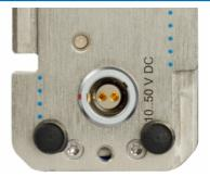
input power supply socket LEMO.1B (female) for a connection with 48 VDC power adaptor (2 guide notches, LEMO.EGE.1B.302)
