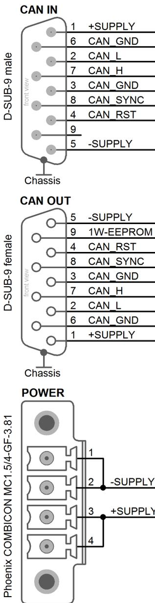
The following overview shows the pin configuration of the CAN-bus sockets (CAN IN and CAN OUT).
