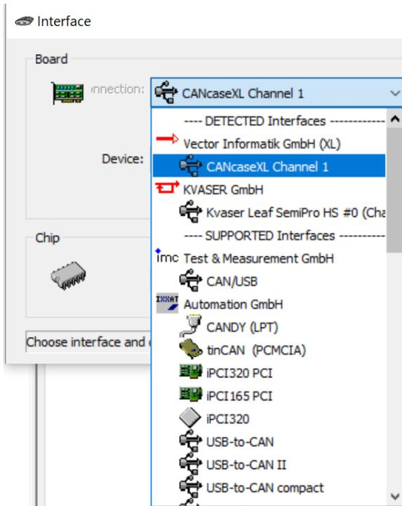
The interface cards supported by imc CANSAS are produced by many companies e.g. imc, KVASER, Vector, PEAK, XXAT and HORIBA. A selection of their installation software is located in the directory `\Driver`.
