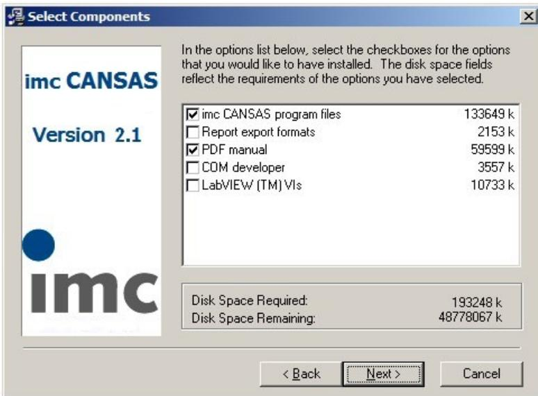
The component Report Export formats only needs to be installed if a imc CANSAS report on module configurations is to be saved in an extraneous format, such as in the form of an Excel file.
