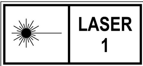
The CANFDX/FBG-T8 device works with class 1 lasers, which means that the device is safe during normal operation. Nevertheless, looking directly into the beam of the Class 1 laser device may cause irritation to your eyesight. This is possible, for example, if the protective cover has been removed or if the device has been damaged in such a way that laser radiation can be released.
