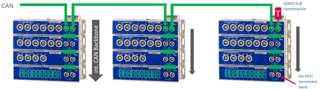
The CAN-Bus is only at the left most module active (side with the visible USB service connection):
