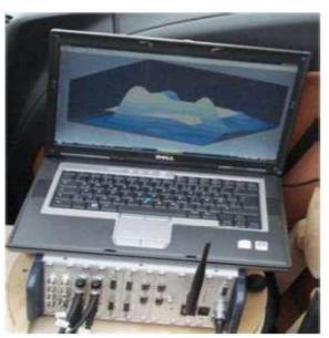
Volkswagen's acoustic analysis system is used throughout the world and in conjunction with imc CRONOS-PL VMS direct, timesaving, economical analysis of the acoustic impact on a car interior.
